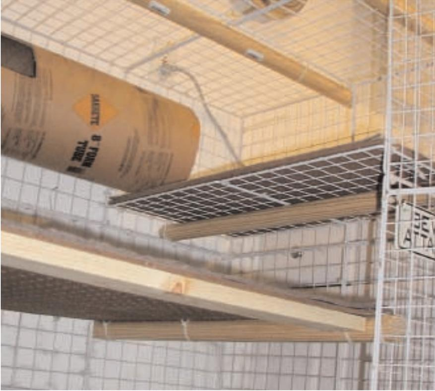
I used closet rod dowels to support the roof and shelves for strength.
